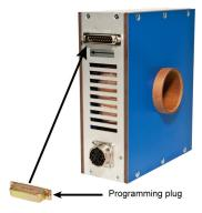
The programming is done by dividing the secondary winding in multiple windings. The programming plug connects the individual windings in series summing up the number of windings to obtain the desired conversion ratio.
