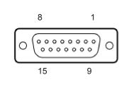
Connect both pins 1 and 9, pins 2 and 10, pins 3 and 11. This will loop the current output to the voltage output module. The sense pins U<sub>s</sub> High Sense at pins 4 and 12, U<sub>s</sub> Low Sense at pins 7 and 14 and the voltage output pins U<sub>s</sub> High Out at pins 5 and 13,  $U_{\rm s}$  Low Out at pins 8 and 15 are internally shorted by rack electronics.
